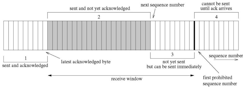
Fig. 2. TCP sliding window
