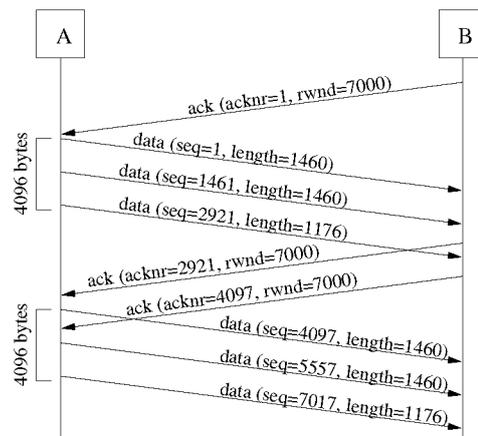
Fig. 5. Block-based buffer utilization
